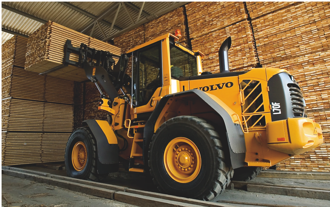
At 168 horsepower and 28,000 pounds, the L70F represents the middle of three model sizes offered by Volvo in the 100- to 200-hp range. For 2007, these Volvo loaders boast a new D6E Tier 3-compliant engine and a new smoother-shifting, quicker transmission.
