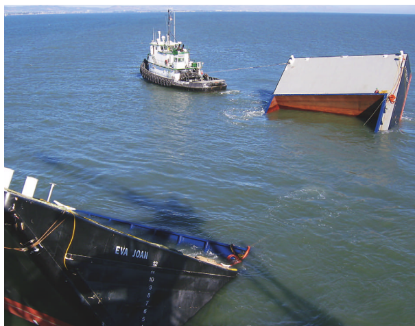
Salvagers dredged tons of sand from the crippled Eva Joan's hold using a pair of 27-hp industrial pumps. The unlikely equipment choice protected the barge's hull from further damage that might obscure evidence of why the vessel failed. Source: ITT Flygt
