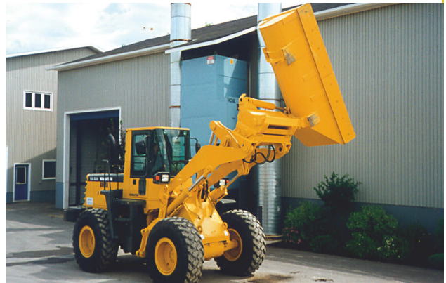
It's still a wheel loader, but the use of such attachments as a side dump bucket can make the carrier more productive.
