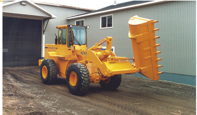
With Craig Manufacturing's Model SDB side dump bucket, placing material exactly where it's needed is much easier.
